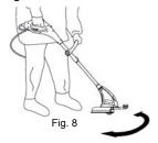
caution: The trimmer line will continue to spin after the On/Off trigger is released. Wait for trimmer line to stop spinning before releasing your grip on the handle.
